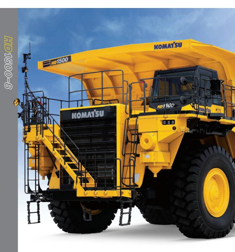
ENGINE POWER 1.175 kW / 1.576 HP @ 1.900 rpm **RATED PAYLOAD** 142 metric tons **BODY CAPACITY, HEAPED** 78 m<sup>3</sup> / 94 m<sup>3</sup>
