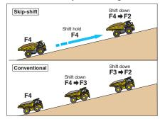
makes the driving smoother, improves the operator's comfort and reduces material spillage.
