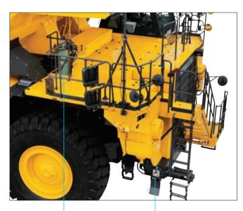
Grease pump pump and reservoir
